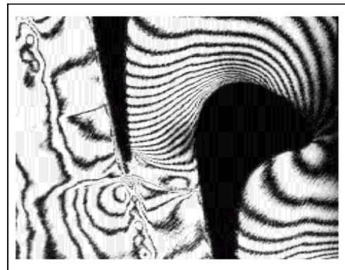
Figure 10. Interferogram of a transonic Flow through a 2-D turbine cascade.
